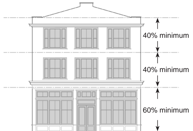
Figure 3-1: Façade transparency requirements for buildings with shopfront.
