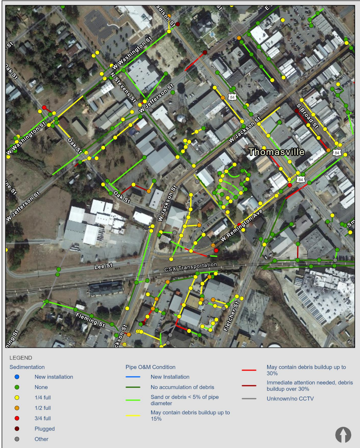
Figure 2.4: Example Results Associated with Sediment/Debris Buildup in Pipes and Inlets.
