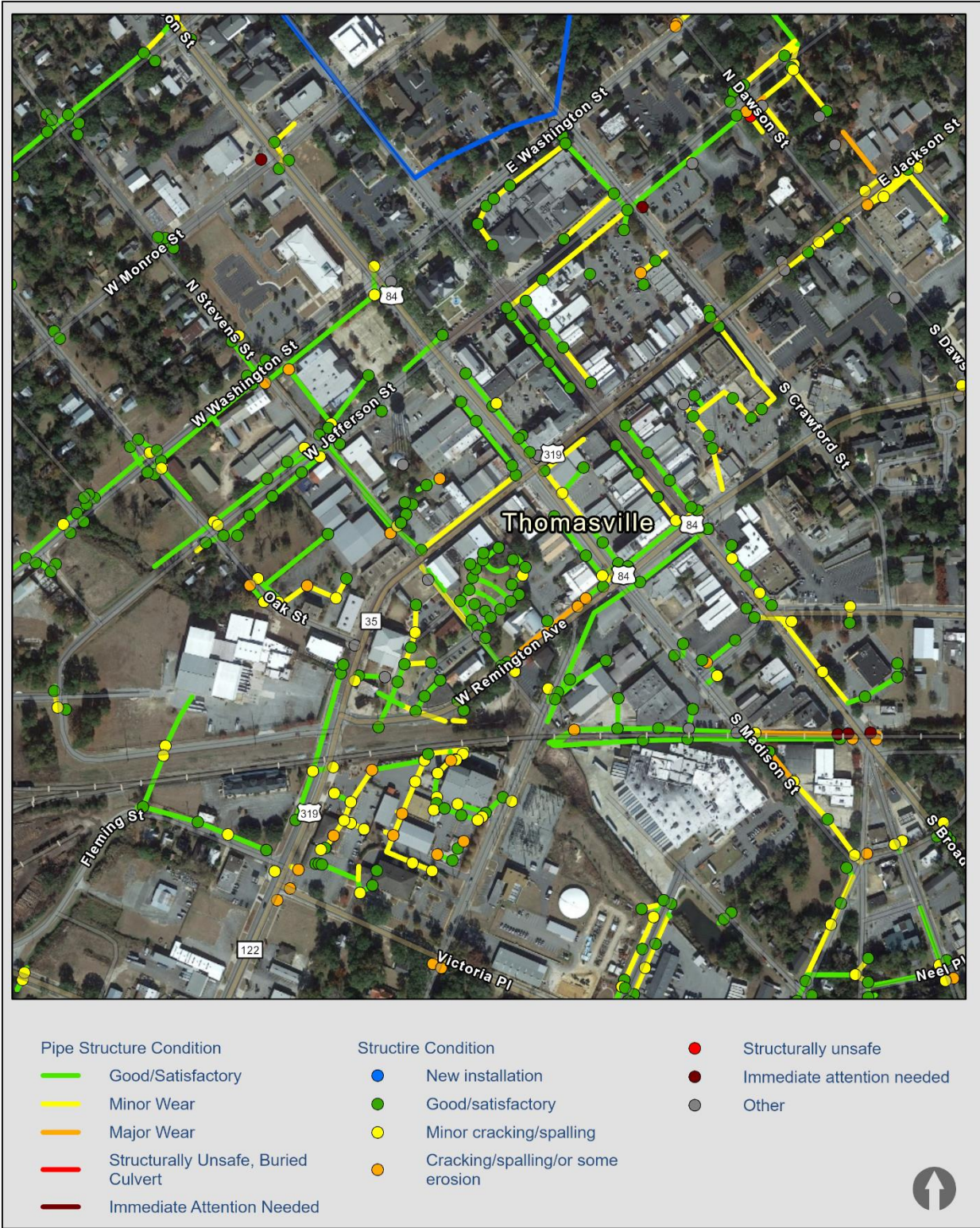
Figure 2.3: Example Results Associated with Structural Damage in Pipes and Inlets.
