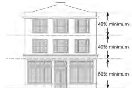
Figure 3-1: Façade transparency requirements for buildings with shopfront.
