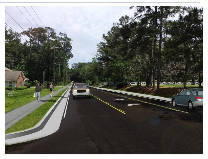
Proposed Two-Lane/Widened Shoulder Typical Section/5 ft sidewalk
