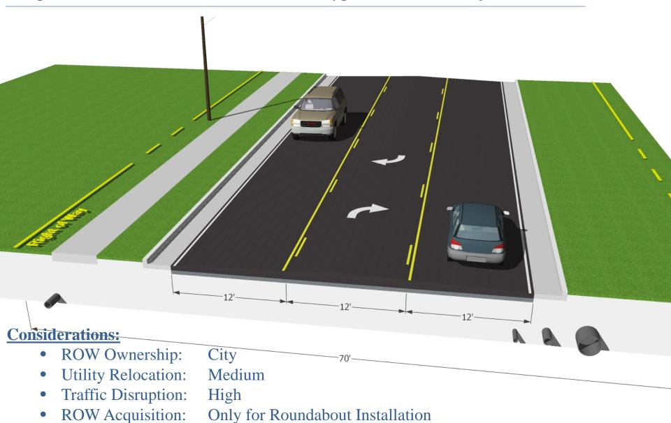
Proposed Continuous Center Lane Typical Section/5 ft sidewalk
